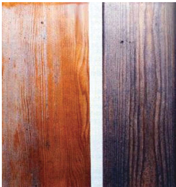
Fig. 5 Wood samples before (left) and after degradation with UV light.
