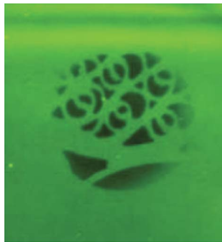
Fig. 7 Fluorescent coating exposed to intense UV radiation through a metallic mask. Dark zones were damaged by the UV radiation.
